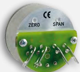
Wiring print with AMP connections
