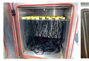
Thermal Endurance to heat and to cold Test
