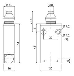
**09** steel end plunger with rubber protection
