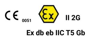
ATEX marking and compliance with harmonised standards EN ISO 80079 (MECHANICAL)
