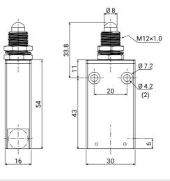
**06** steel end plunger with threaded flange
