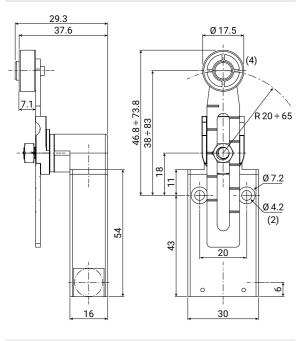
**05** adjustable metal revolving lever and Ø17.5 nylon roller
