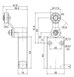
**04** metal revolving lever and Ø17.5 nylon roller
