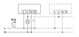
Standard operation with additional control by means of a closing button. If required, the light can be manually switched on or off with the button. To extend the field of detection, the detectors can be connected in parallel.
