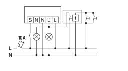
A maximum of 10 devices can be connected in parallel.
