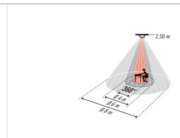
■ Operating area approx. Ø 4 m ■ Head-on to detector approx. Ø 6 m ■ Passage area / diagonally to detector approx. Ø 8 m
