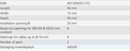
B1, the new on-site mixed concrete range of products for electrical installation work. In addition to the tried-and-tested system features such as the flat front part, sturdy fixing domes and the support element slot with a sprung box base, the new B1 range has innovative conduit entries, sturdy slots for the new B1 Prefix® system wing range, and also bridges – which can be broken out later if required – for connecting accessories in combinations.
