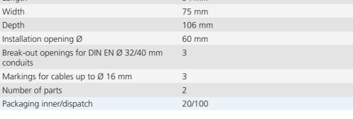
B1, the new on-site mixed concrete range of products for electrical installation work. In addition to the tried-and-tested system features such as the flat front part, sturdy fixing domes and the support element slot with a sprung box base, the new B1 range has innovative conduit entries, sturdy slots for the new B1 Prefix® system wing range, and also bridges – which can be broken out later if required – for connecting accessories in combinations.
