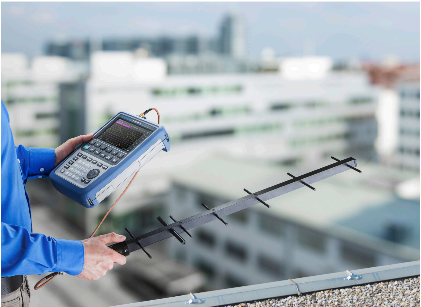
The R&S®Spectrum Rider FPH with an R&S®HA-Z900 Yagi antenna
