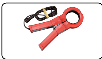
Current Clamp SC 3C 1000A-1V
