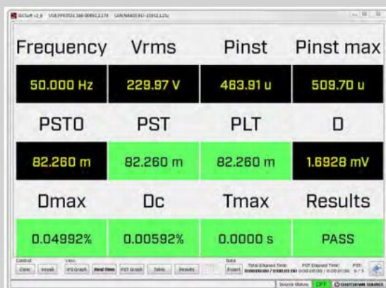
Flicker tests are automatically evaluated against the IEC/BSEN or JIS limits and a pdf/excel report is generated indicated PASS/FAIL.
