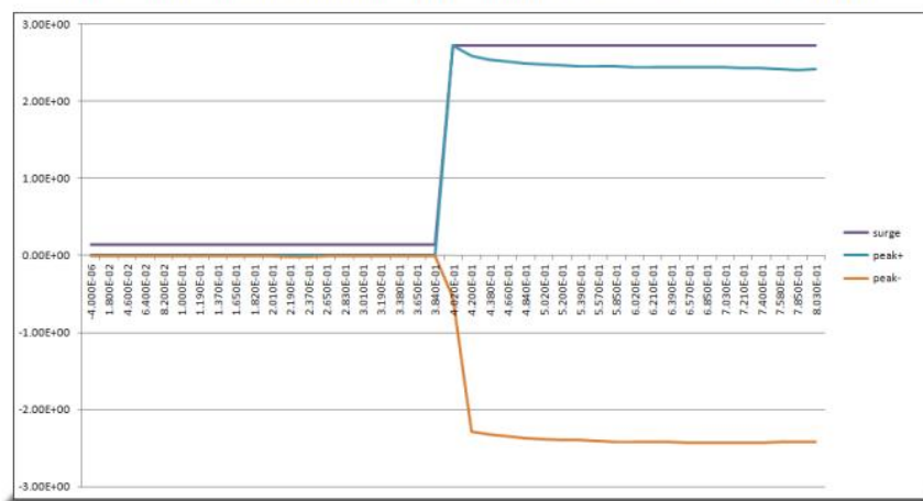
Example Inrush current data, datalogging at nominally 20ms intervals directly to PPALoG
