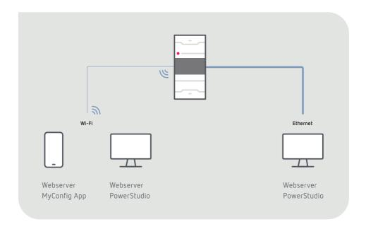
Communicate via ModBus TCP with your energy management software, or integrate it immediately with our PowerStudio SCADA software.
