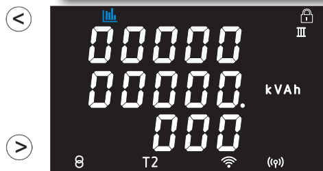
Three-phase Apparent Energy Tariff 2 (5) (kVAh)
