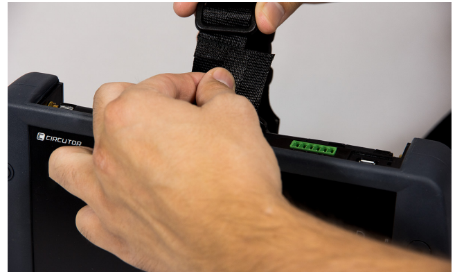
Figure 8: Installation of the fastening strap: Steps 3 and 4.
