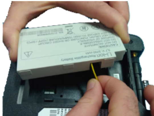
Figure 4:Insert the connection cable inside the battery cover.
