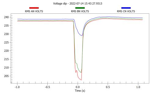
Representation of a voltage dip using PQDiffractor
