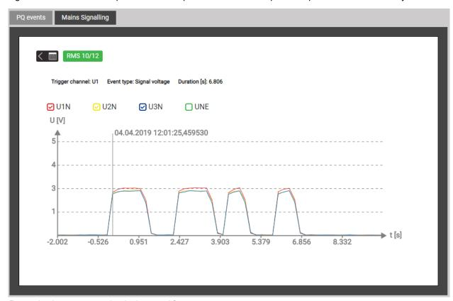
Recognized sequence on the ripple control frequency
