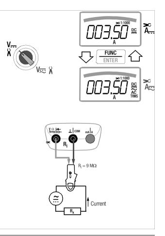
7.7.4 Alternating Current Measurement with Current Clamp Sensors, A AC and Hz  $\,$
