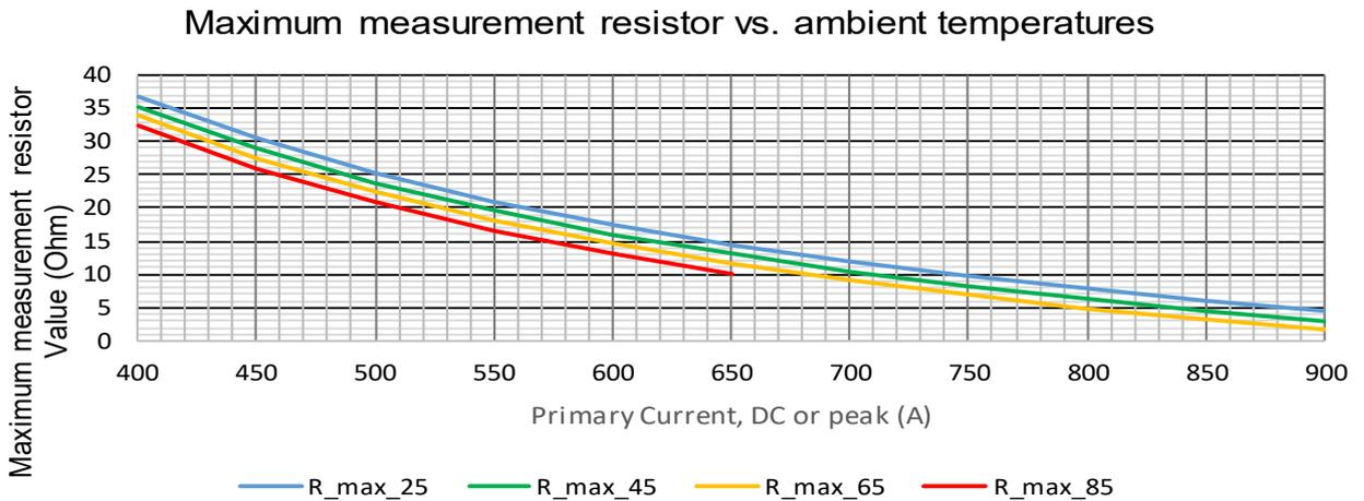
**Frequency and ambient temperature derating (Fig. 2)**
