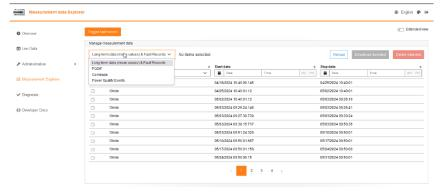
The measurement Explorer can be used to display, download and delete the recording files of the measuring device. Selective filtering allows you to quickly select the files you are looking for.
