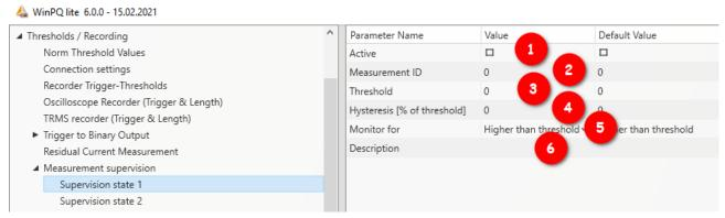
Figure 3: Parameterization of the supervision state
