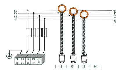
PQI-LV without neutral conductor of current transformer in 4 conductor connection
