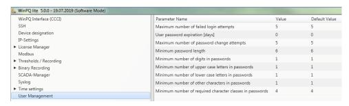
In the menu item User administration parameters, the following necessary parameters can be defined in addition to the password guidelines:
