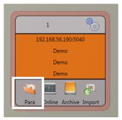
The PQI-LV's parameter setup can be accessed via **Para** button on the device panel. Parameters can be set in basic or expert view, which is also referred to as the classic view in the following sections. These views can be switched by choosing the corresponding selection field in the right main menu of the parameterization window.
