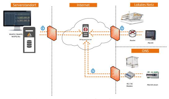
Figure 2: System sketch PQ application with Wireguard VPN (example)
