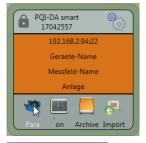
Click on **Para** to download the complete device parameterization from the PQI-LV.
