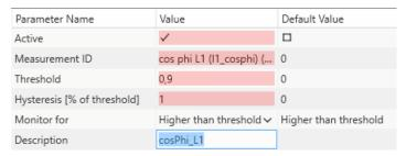
Figure 2: Example for the parameterization to supervise the cos(Phi)
