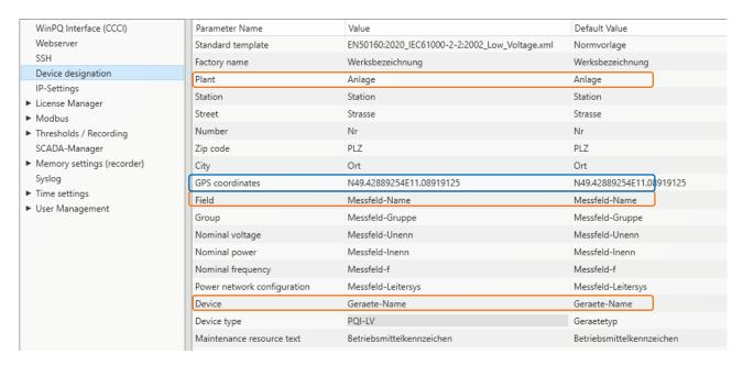
The orange marked fields describe the device tile as well as all fault records and measurement data in the archive.
