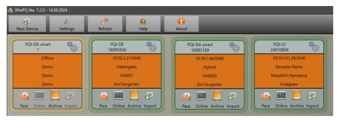
Start screen for WinPQ lite, example with three PQI devices and one offline tile
