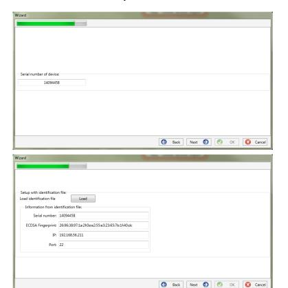
For setup, the serial number of the instrument must be known and entered in the field to establish the first connection via an encrypted connection to the device.
