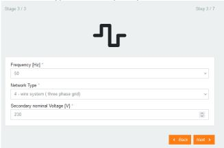
Basic settings for the PQI-LV grid connection Further information on the grid connection can be found in chapter 6.2
