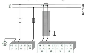
Example of PQI-LV connection with current transformer with small signal output DC mains
