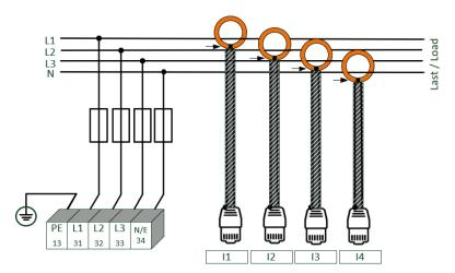
Example: Connection of a PQI-LV in a three-phase - four-wire system
