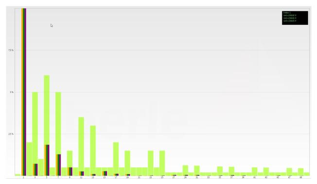
If a harmonic is selected with the mouse pointer, this measurement value is displayed in the field on the top right.
