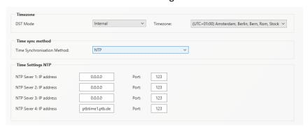
Incorrect time settings can lead to errors or problems during measurement data recording! Using NTP, a good signal quality should be assured (at least Stratum 8)!
