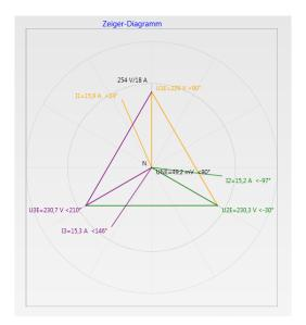
In the vector diagram, connection faults are easy to detect. All phase voltages and currents are displayed with phase angles.
