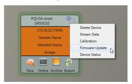
The **General setup** device function tile can be used to carry out a firmware update for the PQI-LV measuring device.
