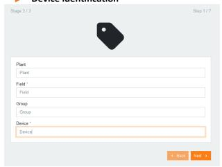
For clear identification of the measuring point, a meaningful designation of the measuring point should be made. These designations are also used for all reports.
