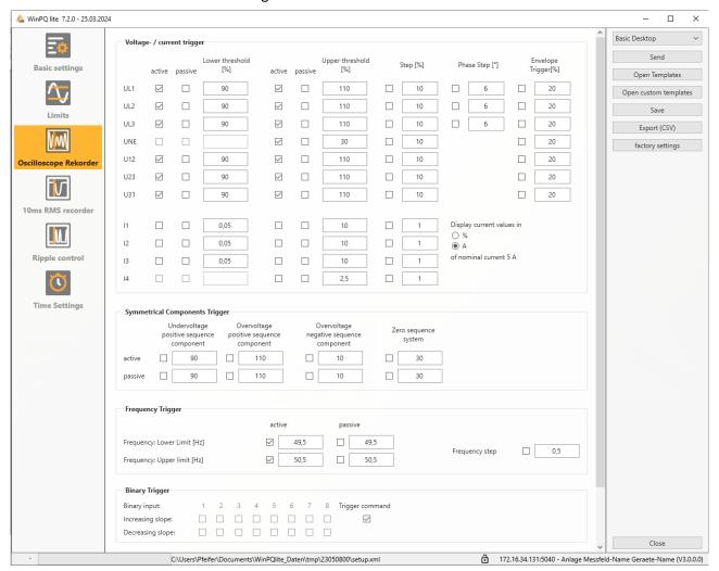
For a clearer overview, all parameters are organized in functional groups. If a field is greyed out and/or not selected, this trigger criterion is not active or cannot be activated. The parameters of the current trigger can be displayed either absolute or as percentage value of the nominal current (setting in the basic configuration).
