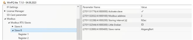
Slaves which are not electrically connected are to be deactivated in the parameterization
