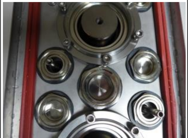
No water is found inside the unit under test around the seal.
