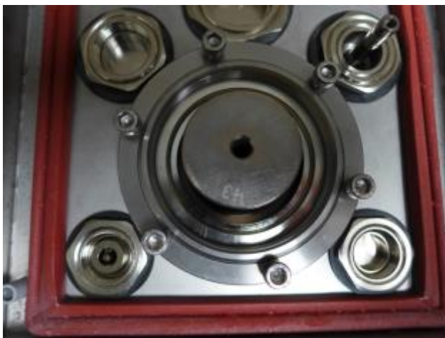
No water is found inside the unit under test around the seal.
