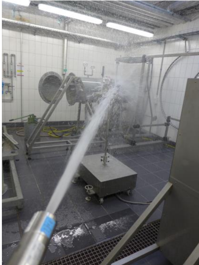
Unit under test during the 3 minutes test with 100 litre per minutes.
