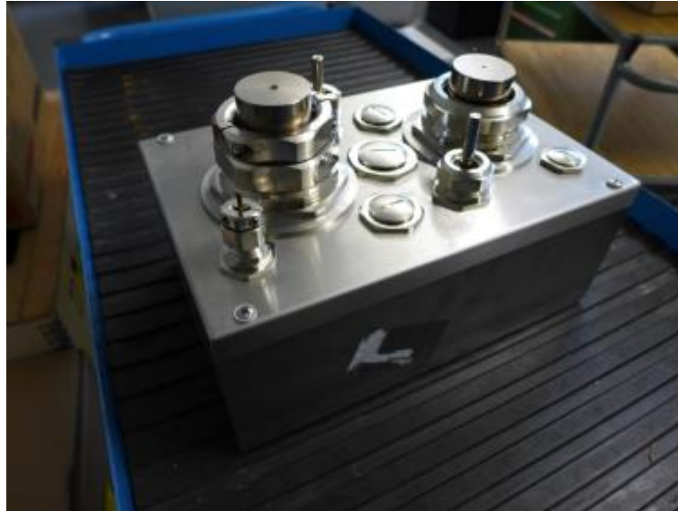
Only the cable glands for ribbon cable are under test.
