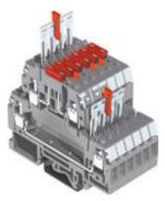
DSFA.4 - detail of the terminal blocks with CNU/8 and SNZ/60 numbering, blade fuse, view of the PTC/4 jumpers on the upper level (upstream the fuse) and on the lower level. The terminal block can be supplied with a nonpolarised LED signal circuit, to detect the fuse blow-out status. Two versions are available depending on the different supply voltages.
