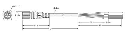
Right-angle XS3F-M422-4 - A Standard cable XS3F-M422-4 - R Robot cable
