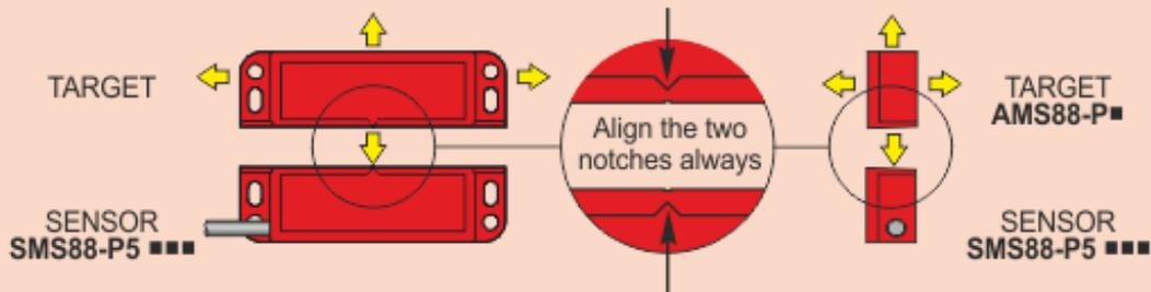
N.B. The minimum distance between *sensor-actuator* systems must be at least 50mm.
