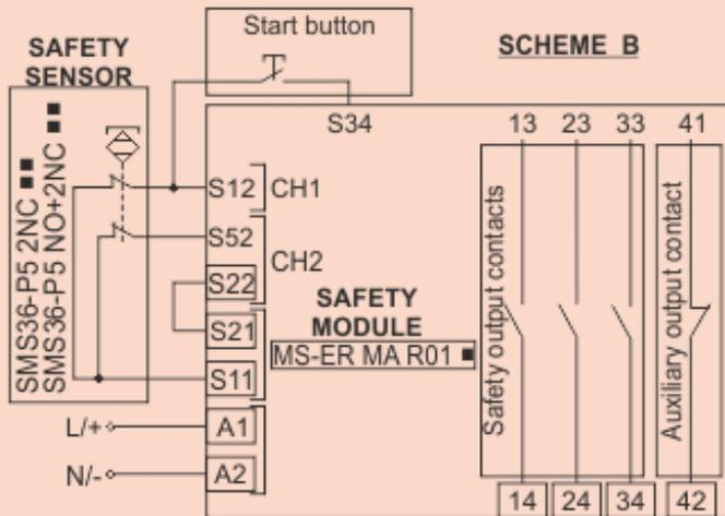
APPLICATIVE CONFIGURATION WITH AECO SAFETY MODULE MS-ER MA R01 ■ SERIES
