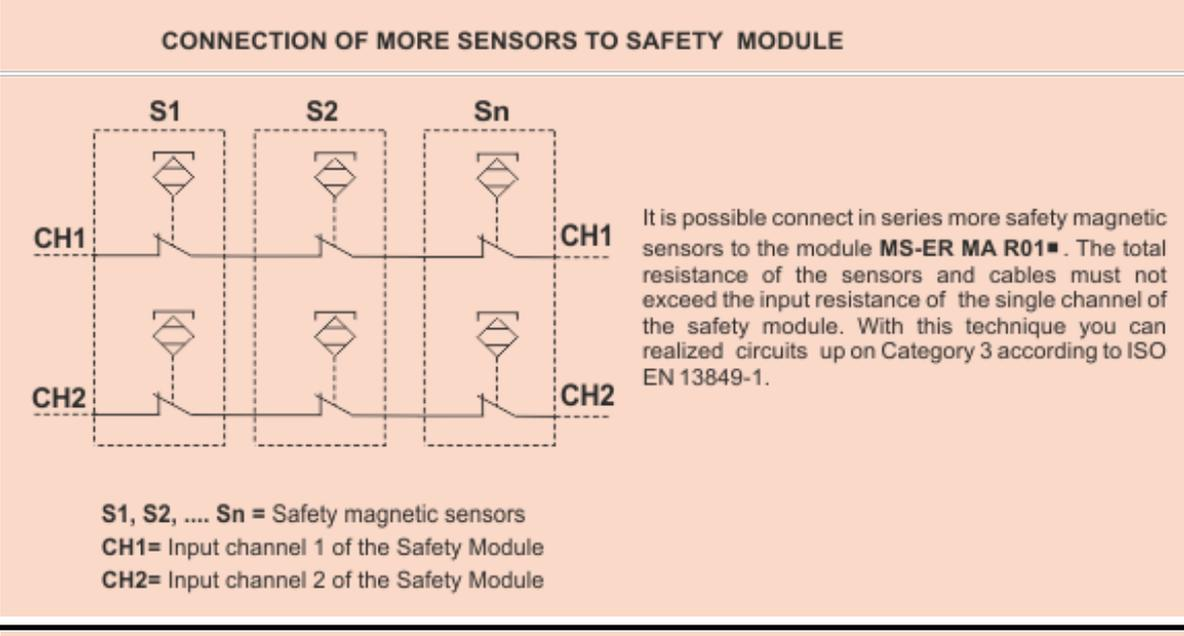
APPLICATIVE CONFIGURATION WITH AECO SAFETY MODULE MS-ER MA R01 ■ SERIES
