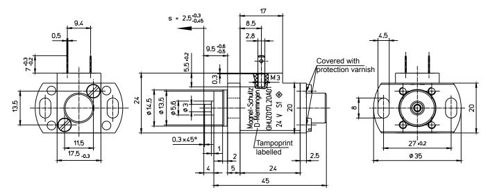
Fig. 3: Type G HU Z 017 L20 A02 / A02 push type (de-energized unlocked) ... A01 with impact damping ... A02 without impact damping
