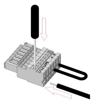
Wire male plug with an adequate cable as is shown by picture, phases order shown on male connector must be kept
