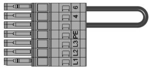
• Bridge from blank pole to pole 6 means input voltage set at 460VAC
