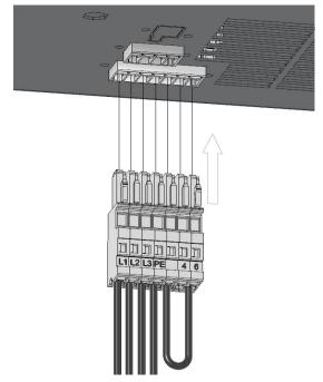
The supply (1) and signal (2) connectors are placed on the bottom of the air conditioner
