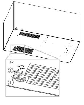
3) Insert signal connector (included in installation kit, refer to picture below) inside of 4 poles female connector placed on the bottom of the air conditioner.
