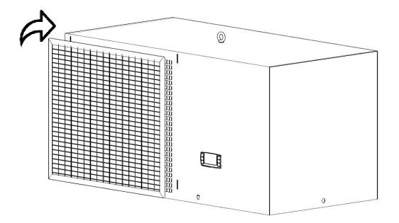
**6.1.1.2** Place the filter on the air conditioner cover as is shown by picture below.
