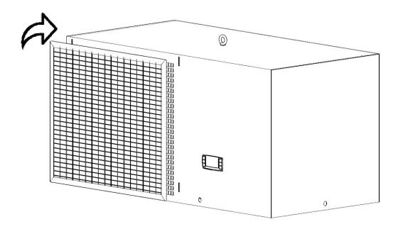
**6.1.1.2** Place the filter on the air conditioner cover as is shown by picture below.
