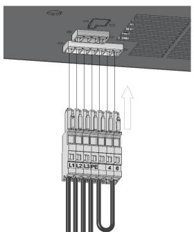
The supply (1) and signal (2) connectors are placed on the bottom of the air conditioner
