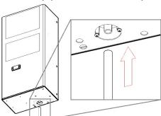
Air conditioner is fitted with condensate evaporator. Condensate is collected into a vessel and it is warmed by the hot discharge compressor pipe. If condensate rises over a certain level, it is evacuated by over flow pipe
