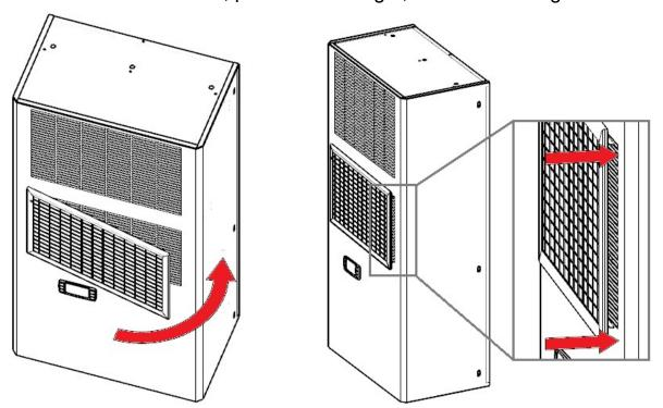
**6.1.1.5** Push the filter to the right until the hooks are right placed inside of grid.
