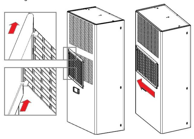
**6.1.1.4** Push the hooks, placed on the right, inside of cover grid.
