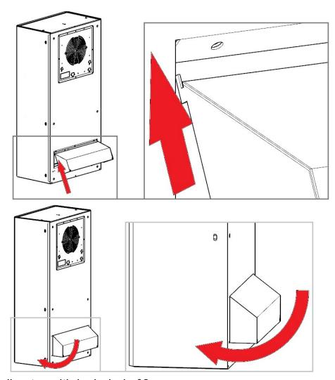
Fix the Flow diverter with included n°2 screws.
