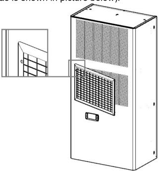
**6.1.1.3** Place the hooks inside of cover grid, start from left side of the grid. Push the filter to the left until the hooks are right placed inside of grid.
