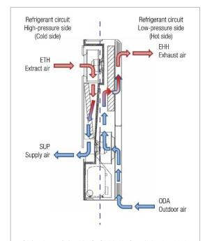
Side view of the KWS-CLM Air Conditioning Unit air guidance. The nomenclature of the air types is according to DIN EN 16798-3 and 12792.
