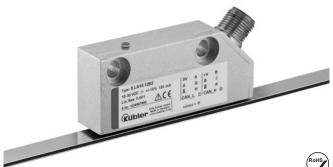
The non-contact absolute magnetic linear measurement system Limes LA10 / BA1 - made up of the sensor head LA10 and of the magnetic band BA1 - reaches a resolution up to 1  $\mu$ m with a maximum distance of 0.2 mm between the sensor and the band (incl. masking tape).
