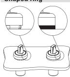
The shaped ring can be used when no label holder or other devices are applied; it prevents dirt and other residues from settling between the potentiometer and the panel or housing.
