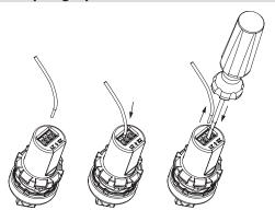
The potentiometer is provided with a three-pole terminal board with PUSH-IN type spring-operated connection. This technology allows a very handy quick wiring procedure. The wire is simply inserted into the appropriate hole, without the need for any auxiliary tooling, through the use of rigid or flexible wires with crimped wire-end sleeve. Release is obtained by pressing the appropriate wire-releasing button.
