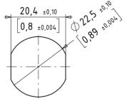
The SENSORswitch is secured against rotation by the illustrated hole.
