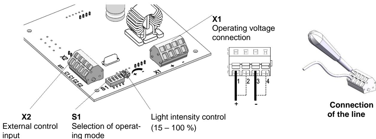
**Note:** Devices with DC voltage are equipped with reverse polarity protection. The function is guaranteed if the polarity of the connections is reversed.
