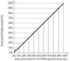
Note: 1. Min. duty cycle of output current is about 8% and the output current is not defined when 0%< Iout<8%.
