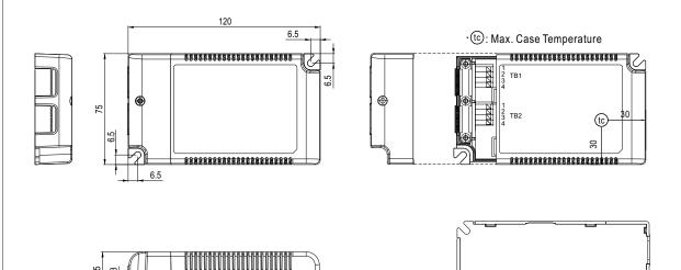
NOTE: Please use wires with a cross section of 0.75~1.5mm² for TB1 and wires with a cross section of 0.5~1.5mm² for TB2.
