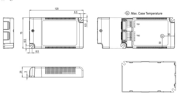
NOTE: Please use wires with a cross section of 0.75~1.5mm² for TB1 and wires with a cross section of 0.5~1.5mm² for TB2.
