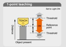
Perform 1-point teaching and the threshold range is set for the distance from the reference surface of the object to be detected.
