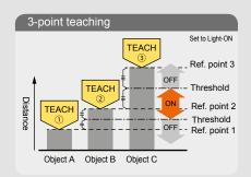
This is the method to set the threshold range by conducting the teaching at 3 points (detecting object A, B and C). After teaching, the reference points are automatically sorted in ascending order (reference point 1, 2 and 3). The thresholds are set at the midpoints between reference point 1 and 2, and 2 and 3, respectively. This is useful for detecting objects at different distances.
